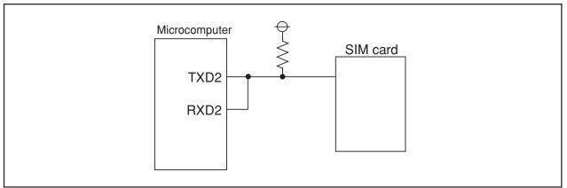
Figure 14.33 SIM Interface Connection
